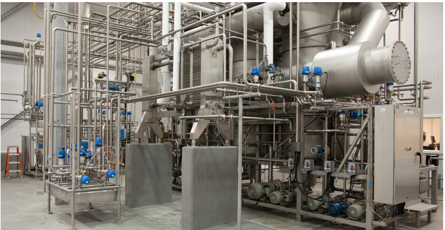
The main condensing unit in the processing plant, which provides significant sustainability benefits.
